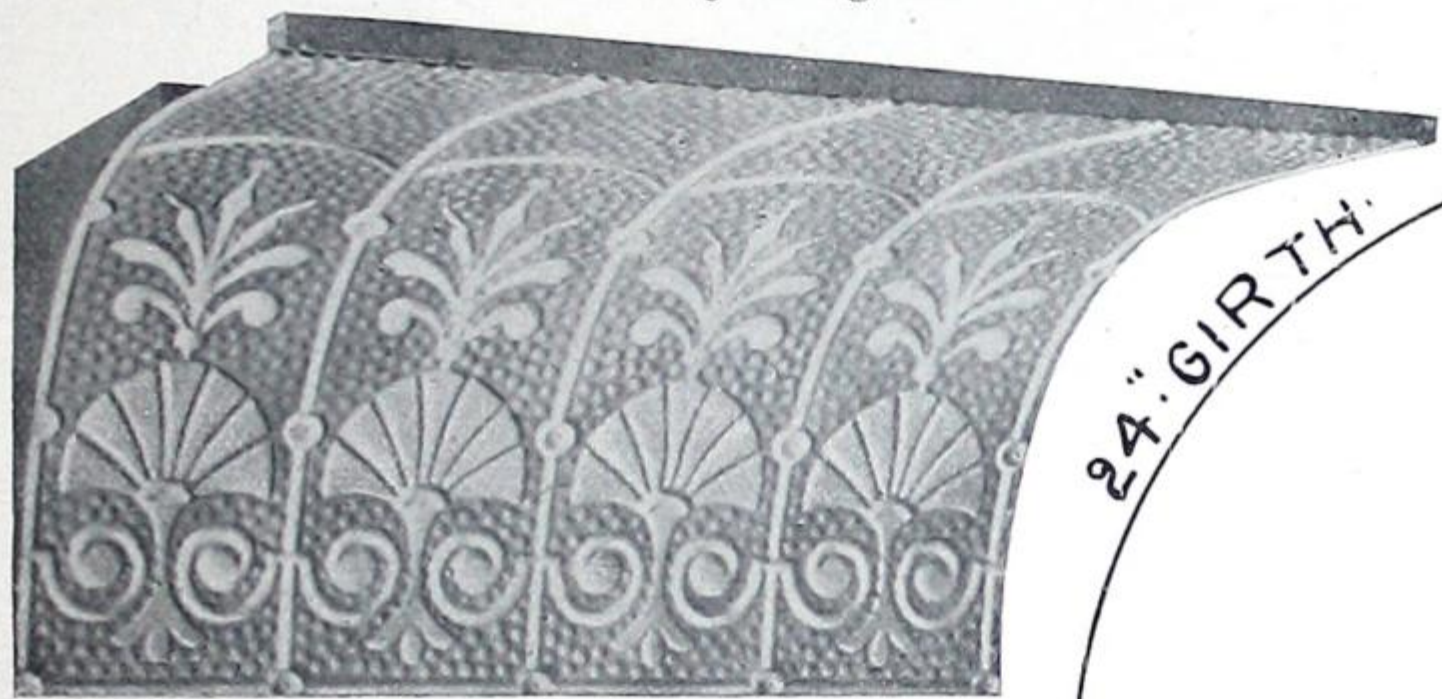
Cove Cornice No. 301.—24-inch girth. Can be supplied any girth from 17 to 24 inches. Use No. 926 moulding for covering mitres on this Cove.
